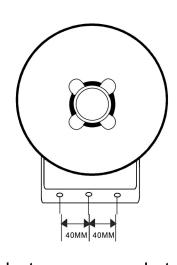
2. The hole in the product bracket corresponds to the hole in the wall and is locked  $\Phi$ 10mm screw, fix the product on the wall, and adjustGood angle
